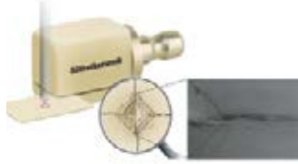
Fig. 4a: SEM image of an indentation in silicate ceramic.
